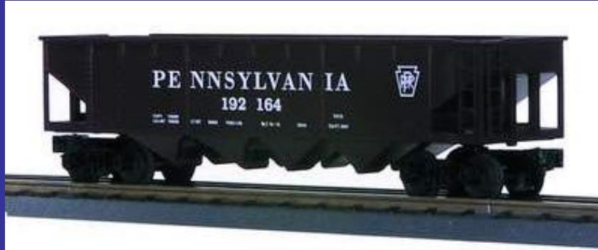
Hoppers look like really tall gondola cars, with two differences. One is that the ends angle out at the top and the other is that the bottom has several V-shapes sticking out between the trucks. This is because hoppers are designed to carry loose materials and dump them out through the bottom. So the angled upper sides help gravity channel the loads out when the spouts in the bottom are opened.
