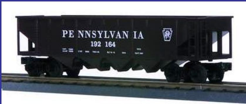
There are two kinds of hoppers, open and covered. The open hoppers are used to haul coal, sand, gravel, woodchips, and the like. Ore cars are shorter-length open hoppers for carrying heavy metallic ores that weigh too much for regular size hoppers. Covered hoppers are used for materials that require protection from weather: grain, plastic pellets, concrete mix, chemicals.
