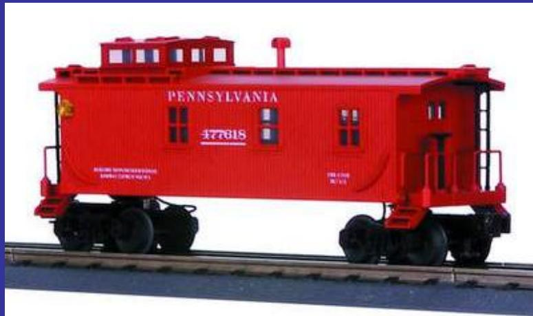
The most famous car in the freight train is the caboose. It served as a rolling office for the train conductor and gave him a place to watch the cars for any trouble and to stop the cars if a coupler broke and the train became separated from the engine. The caboose was often a rough ride, since it came at the end of the train and would get whipped around curves or lurch suddenly to a stop.
