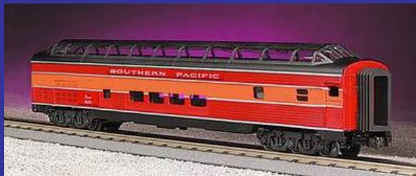
While nineteenth-century wooden cars were beautiful to look at and light to pull, they were dangerous. In wrecks or derailments, cars would collapse, telescoping forward and crushing passengers. Then hot coals from the heating stoves would ignite the cars, cooking anyone who hadn't been crushed. As a result, all-steel cars were developed during the first decade of the 1900s. These cars weighed much more than wood cars, but were much stronger.
