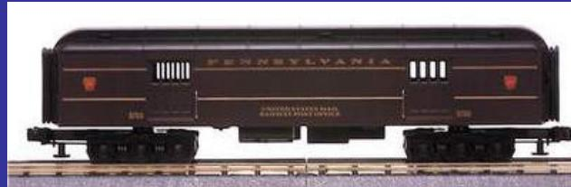
**Head-end cars** are various cars that go right behind the locomotive, and carry packages rather than passengers. The most important of these is the *baggage car*, which holds passengers' luggage. Trains sometimes used combine cars which had a baggage compartment up front and passenger seating area in the rest of the car. Often these cars were designated smoking areas.
