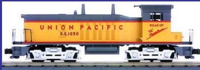
While switchers are small engines that are most often used in rail yards to move cars from one track or shed to another, road switchers are slightly larger and more flexible engines (1500 hp or more) that are small enough to perform yard duties but powerful enough and equipped to carry loads at speed on the mainline, too.
