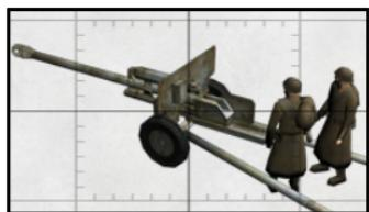
The ZIS-3 was initially intended to be a field gun, but its 76.2mm caliber made it a prime weapon to use in the anti-tank role. It replaced the ZIS-2 early in the war, and became the most numerous field gun in the Soviet Army. In all, over one hundred thousand were built.
