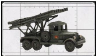
Named for a popular Soviet wartime song, the Katyusha was developed in response to the Nebelwerfer rocket launchers the Germans pressed into service. Trucks outfitted with this launching system had between 14 and 48 tubes attached.
